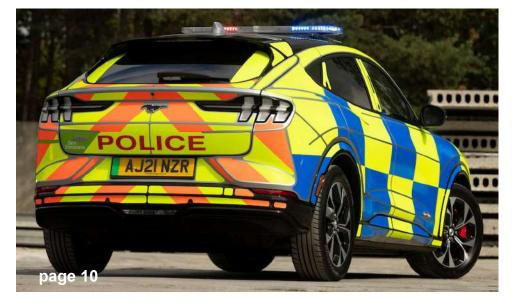
"The vehicle range is uncompromised as the blue light equipment is being drawn from the vehicle's 12V battery and not the drive battery," says Terry Adams, manager of sales to police services in the U.K. "In future developments, we will look to increase this battery capacity to allow for additional equipment to be fitted."
