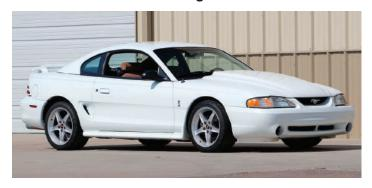
Although the 1971 Boss 351 was the final Mustang with solid lifters, it wasn't the final 351-powered pony. In 1995, SVT brought back the 351 to power its second Cobra R model. The engine was fuel injected and featured a 9:1 compression ratio. It made 300 hp, which was considerable at the time, and was backed by a Tremec five-speed. Only 250 were built. Motor Trend tested one, hitting 60 mph in 5.2 seconds.
