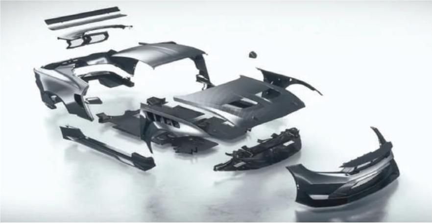
The fenders, hood, cover that replaces the trunk lid, door sills, front splitter, rear diffuser and roof are all carbon fiber with optional carbon fiber front and rear fascias. An available aero package that includes a comprehensive underbody aerodynamic tray is also executed in carbon fiber.
