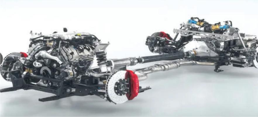
The rear-mounted 8-speed dual-clutch transaxle and lightweight carbon fiber driveshaft contribute to near-50/50 weight distribution for the Mustang GTD.
