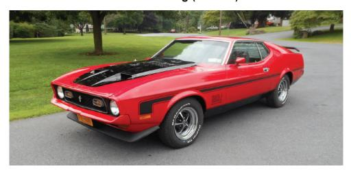
The 1972 Mustang 351 HO was yet another example of Ford managing to slide one or two decent performers in beneath the nose of the EPA, as 1970s emissions mandates were enacted. This particular Mustang served largely as a low-compression, detuned version of the Boss 351. Though its output had effectively been limited to just 275 horsepower, the 351 HO still had much to offer.
