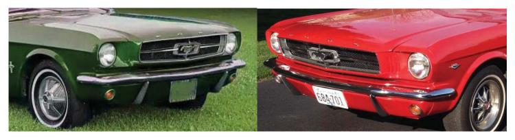
Even if you find a stiffening edge though, it doesn't absolutely verify that you're looking at a '64. The other external marker many look for are the hood moldings. The '64.5 Mustang typically doesn't have the hood moldings that are seen in '65 Mustangs.
