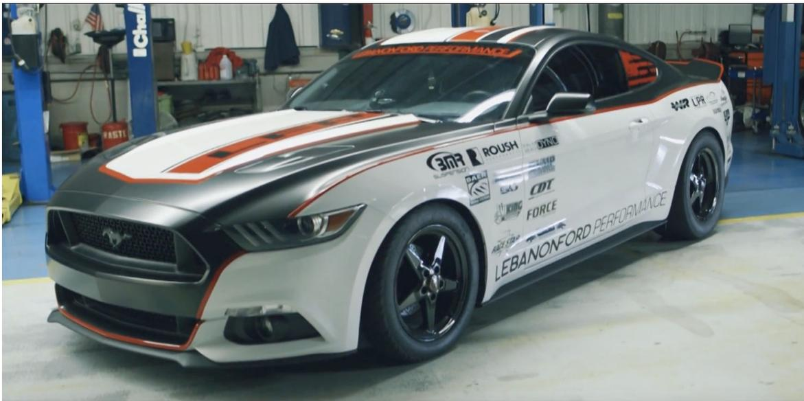
Lebanon Ford also adds Viking adjustable shocks and BMR springs tuned for drag racing, and installs a set of Mickey Thompson tires on 17x5-inch front, 17x10.5-inch rear wheels. The LFP 10 also gets a bolt-in roll cage to keep the NHRA happy, and upgraded drive- and half-shafts to cope with the extra power.
