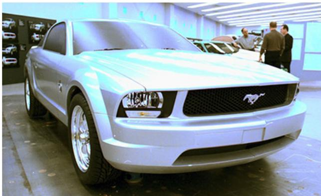
*The overall shape of the 2005 Mustang front fascia is now near final by late 2001 although this clay model still has large round headlamps with turn signals integrated. By production the turn signals would move into the bumper.*
