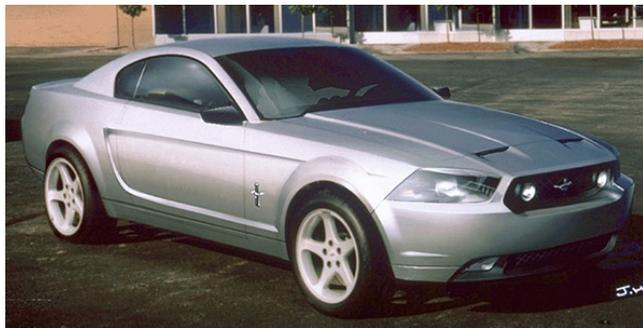
*An early computer rendering that looks like a heavily modified 4th generation Mustang with the longer wheelbase first seen on the 1999 Ford Racing FR500 demonstrator. A forward-leaning shark-nose grille and side hockey-stick similar to the production 2005 model.*
