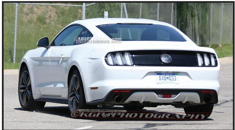
The taillight changes, however, go a bit deeper than simply the color of the unlit taillights—they function differently than our U.S.-spec taillights. Instead of the Mustang's sequential rear-turn indicators, these signals alternate between two red bars using the taillights' inner LED strips, and a single amber strip on the outer light bar.
